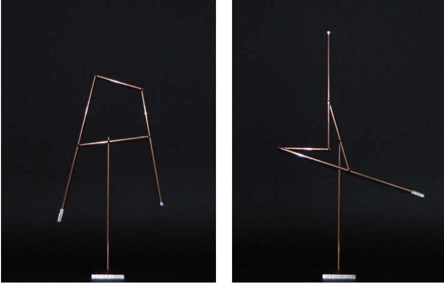
Fig. 2.17 Physical model in two poses of the force-balanced four-bar linkage in Fig. 2.14b when f_i = 0 . (see model in motion at: www.kineticart.nl )
