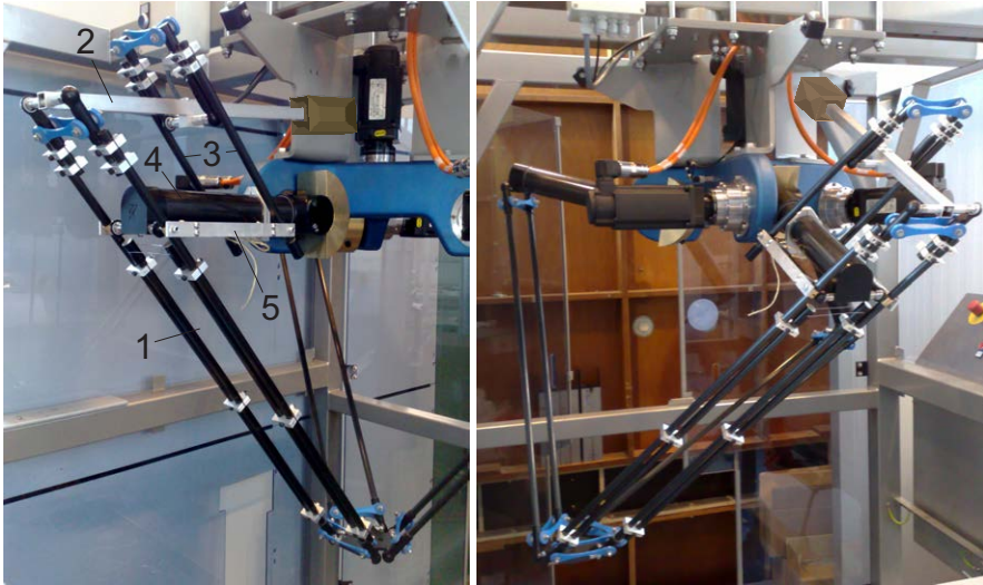
Fig. 3.41 Force-balanced Blueprint Automation delta robot of which one arm is a spatial 3-DoF pantograph with a counter mass on elements 2 and 4. Parallelogram 3 remains parallel to parallelogram 1 with a torsion bar 5 on each side of the actuated element 4 with which the rotational motions of parallelograms 1 and 3 are synchronized. (patented [100])
