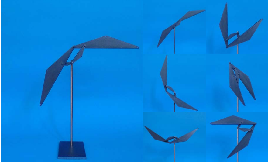
Fig. 2.21 Physical model of the force-balanced pantograph linkage in Fig. 2.20b in various poses. (see model in motion at: www.kineticart.nl )
