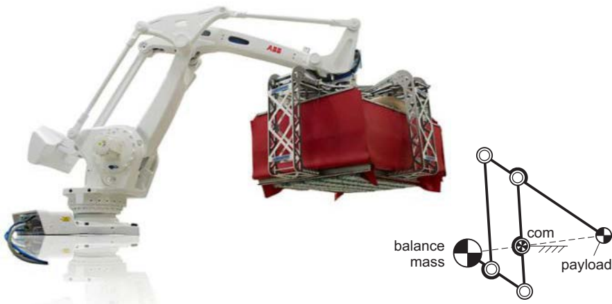
Fig. 1.5 ABB IRB760 palletizer manipulator with balance mass for force balance of manipulator and payload to have low dynamic forces in the base, increased payload capacity, and increased efficiency and safety. (www.ABB.com, 2014)
