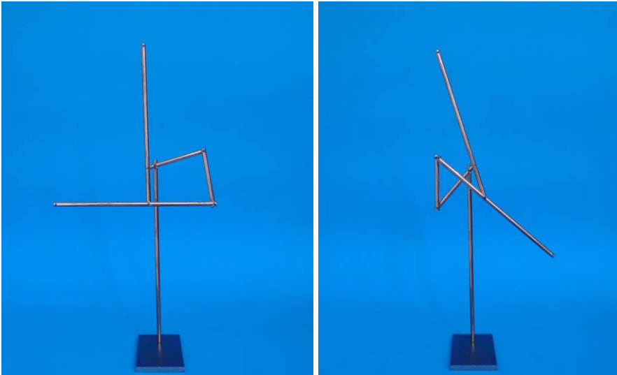
Fig. 2.18 Physical model in two poses of the force-balanced four-bar linkage in Fig. 2.15 when f_i = 0 . (see model in motion at: www.kineticart.nl )
