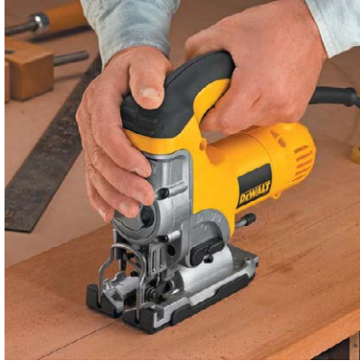
Fig. 1.6 For high-speed hand-held tools dynamic balance improves ergonomics, reduces the risks of injuries, and improves the quality of the work. (balanced jig saw DW331K, www.dewalt.com , 2014)
