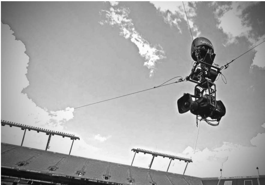
Fig. 1.9 The Skycam robotic camera system consists of a cable driven parallel manipulator with a camera system as end-effector that is dynamically balanced for stability. (www.skycam.tv, 2014)
