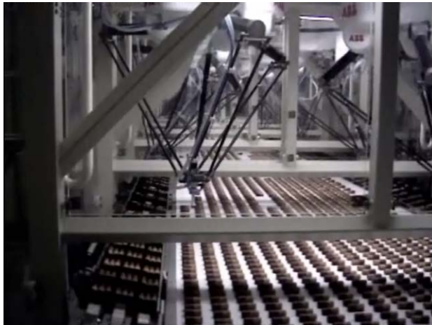
Fig. 1.1 To mount high-speed robotic manipulators, heavy supports with large footprints are required to resist the high shaking forces and shaking moments in the base. (ABB Flexpicker Delta robot)
